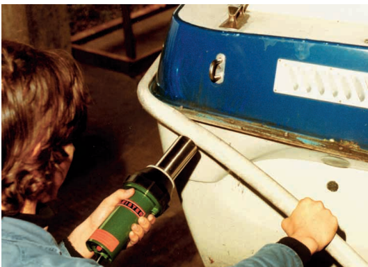
Fitting of a PVC sheer rail to a boat with the ELECTRON.
