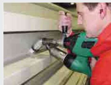
The 45° angled adapter for the WELDPLAST S2 facilitates welding in difficult positions. (accessory)
